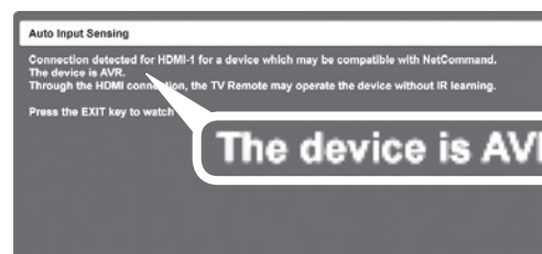
Figure 2. TV recognizes the CEC device. The TV's NetCommand for HDMI is on and the connected device's HDMI Control is also on.
